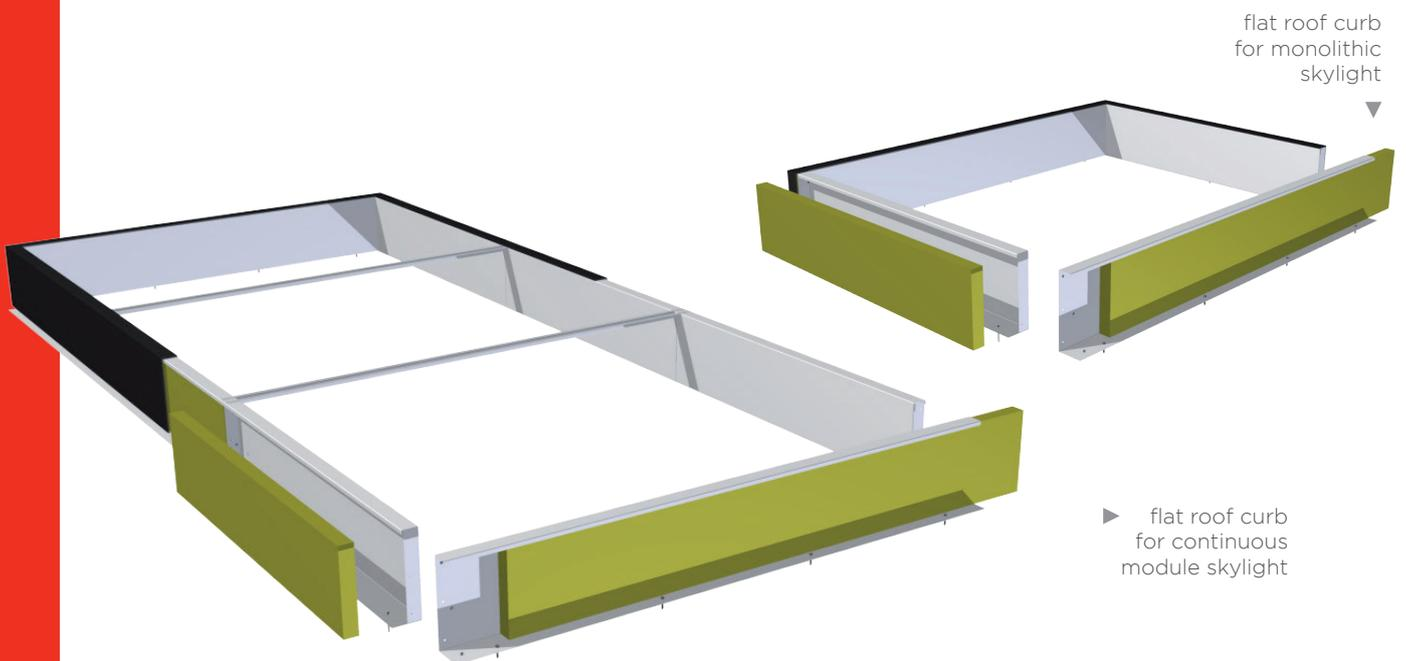
Curbs, designed to be assembled on-site, for installation on flat roofs, are made of C-section steel sheets with chromatic finishes. The height and polyurethane insulation panel can be customised based on project requirements. The curb is designed in 3D to accommodate both monolithic and continuous skylights, ensuring efficient packaging and transportation. Fittings and step-by-step assembly instructions are always provided.
