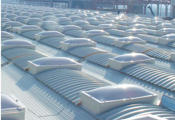
Curbs, to be assembled on-site, for coupling with insulated curved sandwich panel roofs made of steel sheet with chromatic finishes. The height and insulation panel in polyurethane can be customised according to project requirements. The curbs are shaped to allow for overlapping with the roof on two sides while being supported by the beams on the other two sides.
